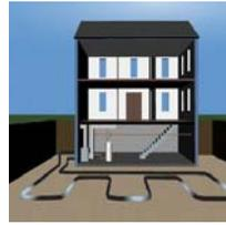
Geothermal energy utilizes an electric ground-source “heat pump” and the temperature of the earth or groundwater to store and harvest heat. A “closed-loop” system circulates water or liquid
