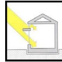
In “Passive” systems, the mass contained in the building materials absorbs and re-radiates the solar heat in the occupied spaces. Concrete slabs, tile, masonry and extra-thick drywall or plaster
