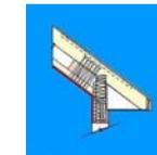
The building shell uses advanced framing techniques to incorporate air-sealing details, reduce construction materials and allow for high insulation
