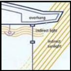
Natural lighting techniques allow a significant reduction in the cost and amount of artificial lighting.
